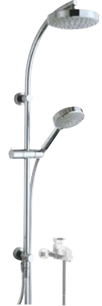
SHA-1217R* Exposed Shower Pipe with Provision For Simultaneous Working of Showers with Operating Divertor Knob, Round Shape ø24mm, Size 975X370mm with Sliding Holder For Hand Shower, Wall Bracket & 8mm dia, 1M Long Flexible Tube (for connection to Exposed Shower Mixer) Without Shower Rs. 12,500
